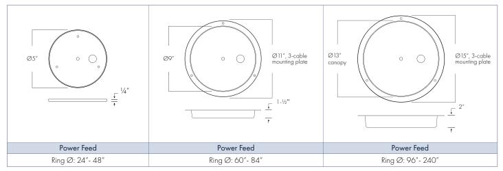
MCC canopy illustrations are shown with 3-cable mounting plates, please note  $\emptyset$  greater than 72" will have 6-cable mounting plates.
